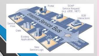
ESB is a pattern whereby a centralized software component performs integrations to backend systems (and translations of data models, deep connectivity, routing, and requests) and makes those integrations and translations available as service interfaces for reuse by new applications. The ESB pattern is typically implemented using a specially designed integration runtime and toolset that ensure the best possible productivity
